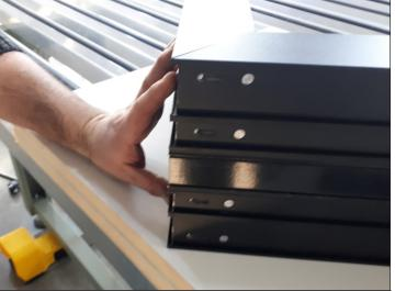
Step 12: After tightening the corner brackets, make sure that all the bracket balls are in their assigned places of the corner. In case one of the balls has fallen out, unscrew the bracket screw, and use the hex key to place the ball in its desired position and to screw back the corner bracket;
