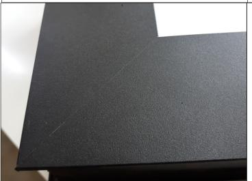
**Step 15:** The corner must be properly aligned. We will repeat all the above instructions for the other 3 corners of the frame;
