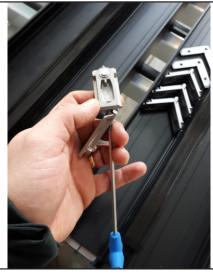
**Step 3:**Open each tightening angle bracket to the maximum (unscrew the bracket screw using the hex key);
