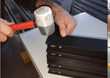
**Step 11:** Align the corner (using a rubber hammer) until you get the desired result, and afterwards tighten all the corner brackets to the maximum;
