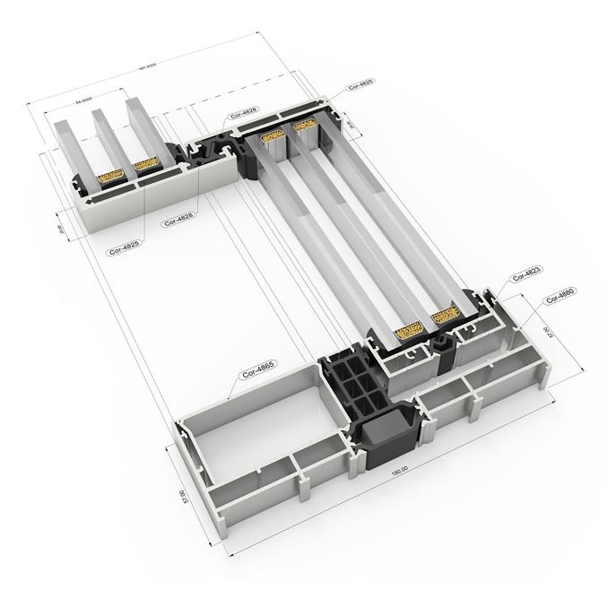
The Panarama Star system is a high-performance aluminum minimally framed large patio sliding system. Its designed for stunning aesthetics, comfort and quality, durability, energy performance and security.
