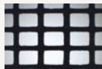
Conventional window screen (11 mils diameter)
