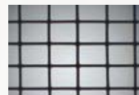
Gore inLighten window screen (5 mils diameter)
