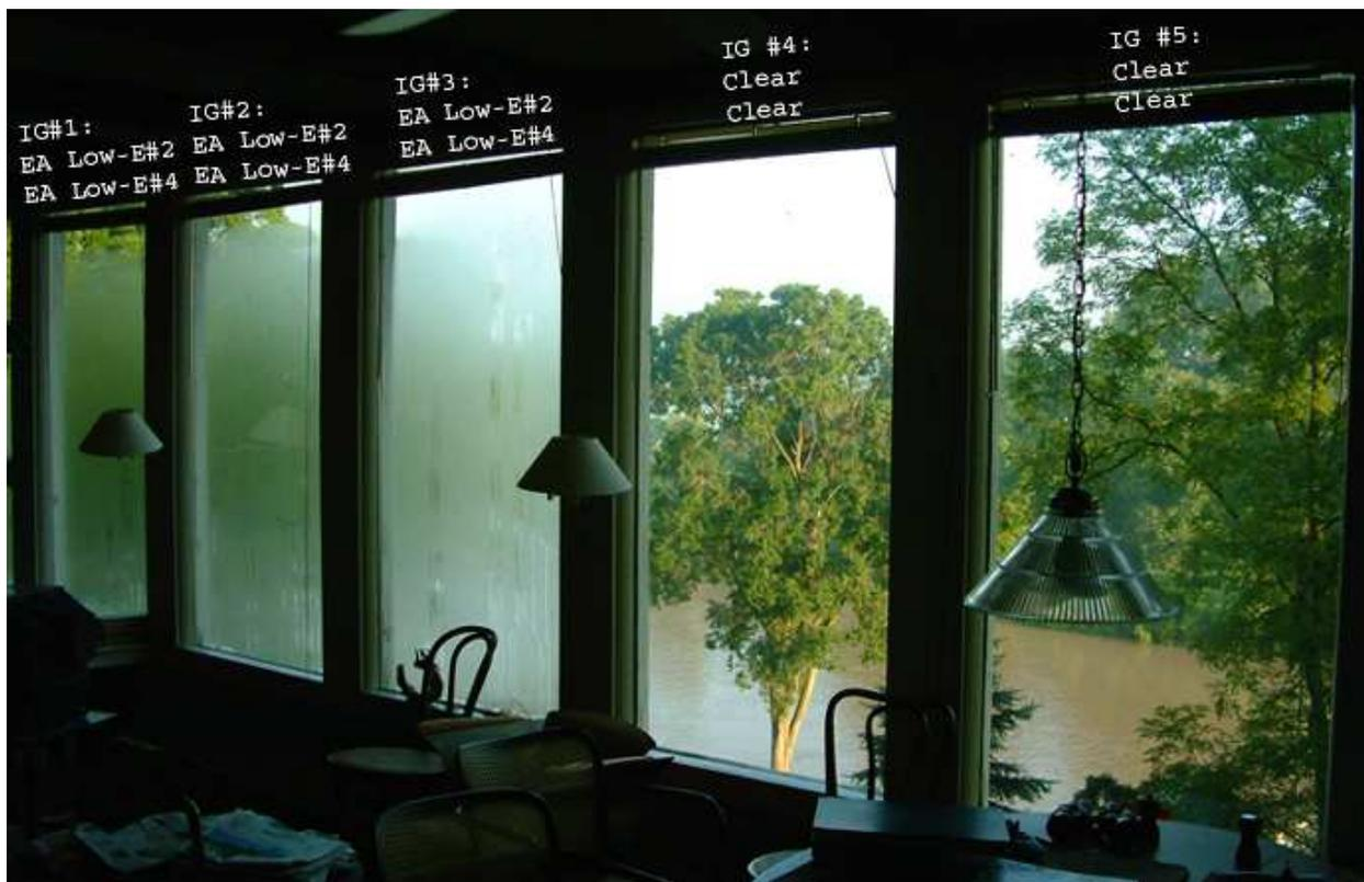
First surface condensation on 3 high performance North elevation, river facing, windows, Ohio, 7:30 a.m in June. Still air, 70 °F, 85% Relative Humidity, 65 °F Dew Point. No air conditioning.
